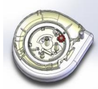
Assembly of counter wheel and idler gear
