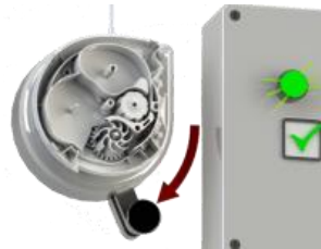
Activation of the device to check the gear box function
