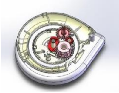
Assembly of drive-, base and index wheel
